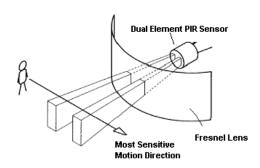
Fig2 Sensitivity detection of PIR Detector
